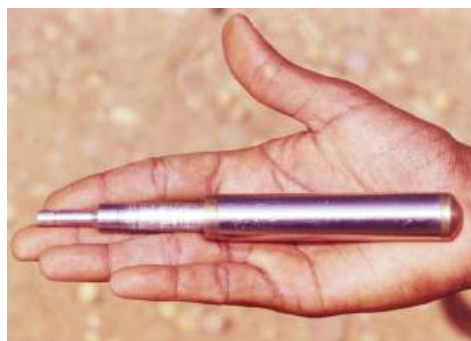
A penetrometer: a device used for quality testing of CSEB
