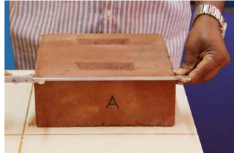
Dimensions of CSEB block being checked for quality control
