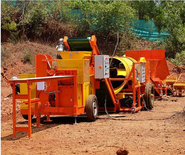
Auram press 3000- used to produce CSEB Blockl
