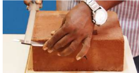
Dimensions of CSEB block being checked for quality control
