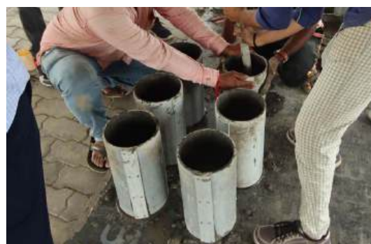
Casting PEC samples on site
