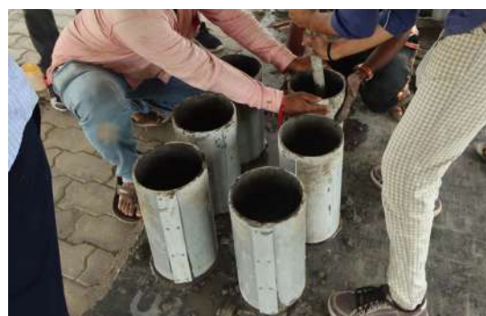
Casting PEC samples on site
