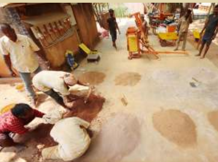
Combining the red gypsum with various mix ratios
