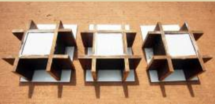
Shrinkage tests being conducted on three cube samples
