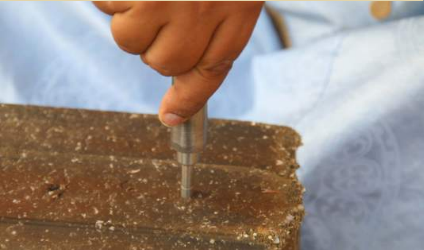
Testing CSEB produced by a motorized block press in Sélibaby
