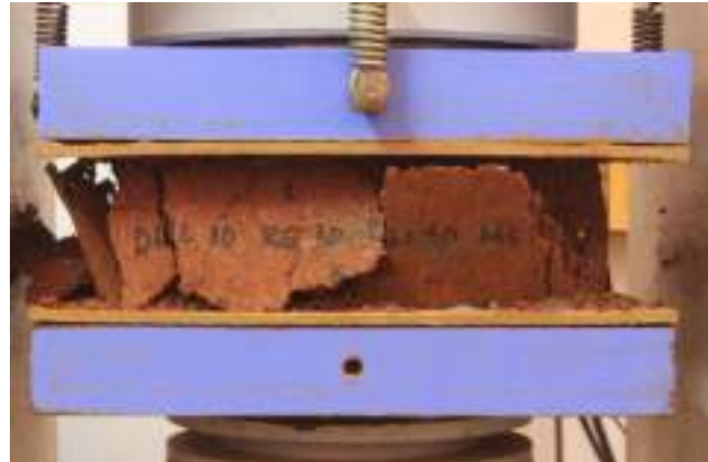
Testing a CSEB with red gypsum
