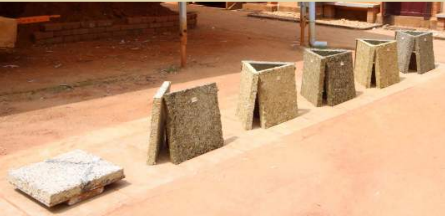
Sample insulation panels drying
