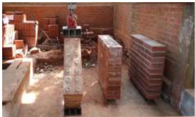
All three wall assemblies to be tested
