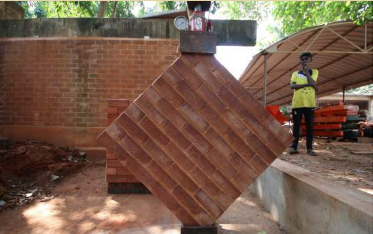
An Innobloc 250 wall assembly undergoing a shear test at Aureka
