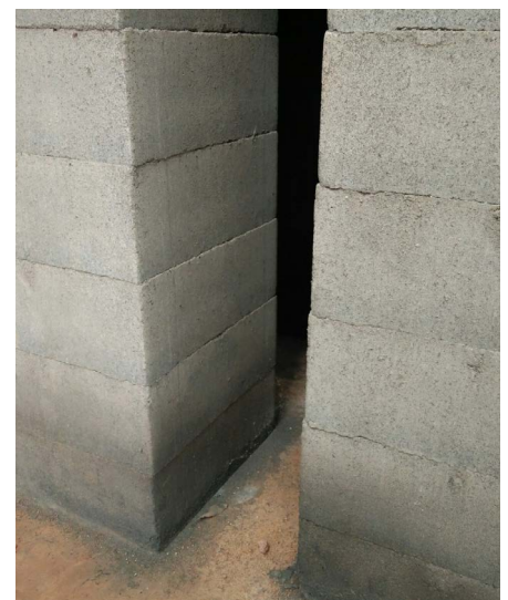
Foundry sand blocks awaiting testing
