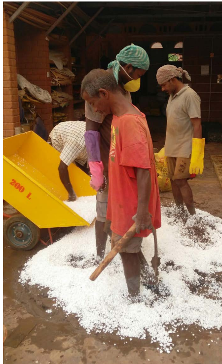
Mixing shredded polystyrene with water, soil, and cement ; various finished samples
