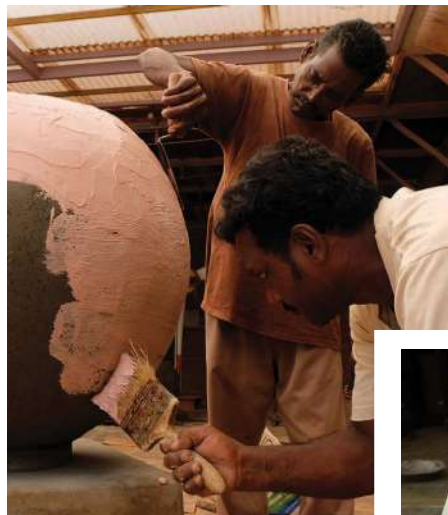
From top to bottom: preparing the wire framework for the planters, the framework covered with chicken mesh, applying the ferrocement mix with a trowel, adding a thin basecoat and burnishing it with a stone, and one of the completed planters curing
