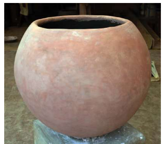
From top to bottom: preparing the wire framework for the planters, the framework covered with chicken mesh, applying the ferrocement mix with a trowel, adding a thin basecoat and burnishing it with a stone, and one of the completed planters curing
