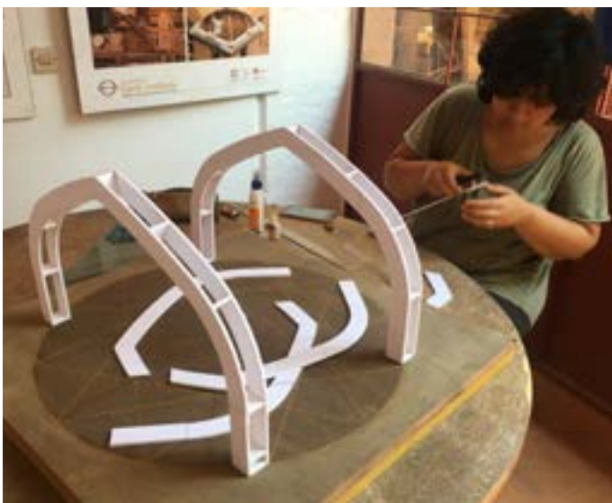
Tiny adobes for the models ready for use; Behnaz working on the "Karbandi" dome formwork; Pouya testing out the adobes
