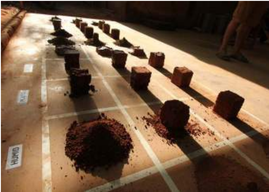
Demonstration of Carazas Test during the Bioclimatic Earth design workshop
