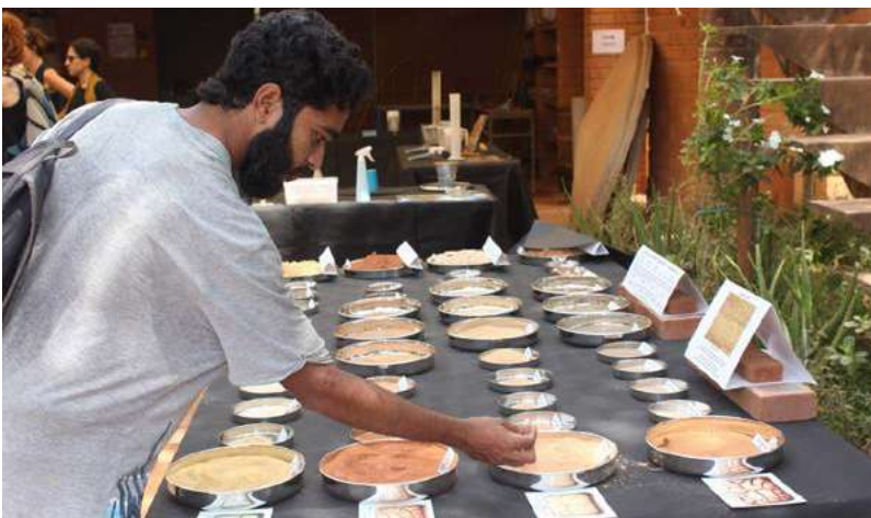
Four Auroville soils were carefully sieved and displayed to show their composition according to grain size.
