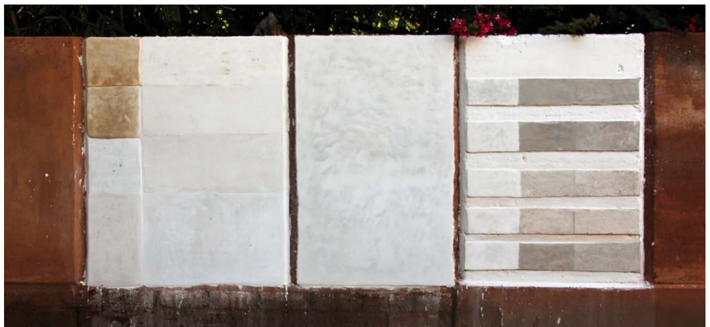
Panel 3 (Left) - Shell and Village Lime Tadelakt | Panel 2 (Middle) - Industrial Lime Marmorino | Panel 1 (Right) - Industrial Lime Plasters
