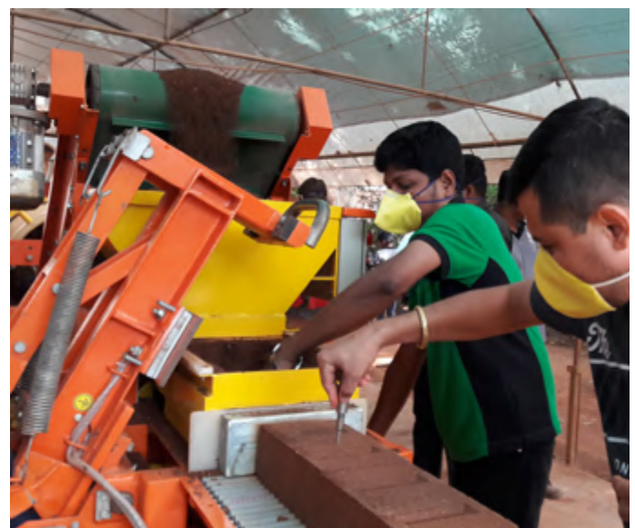
Using the semi-automatic Auram 4000 to make CSEB
