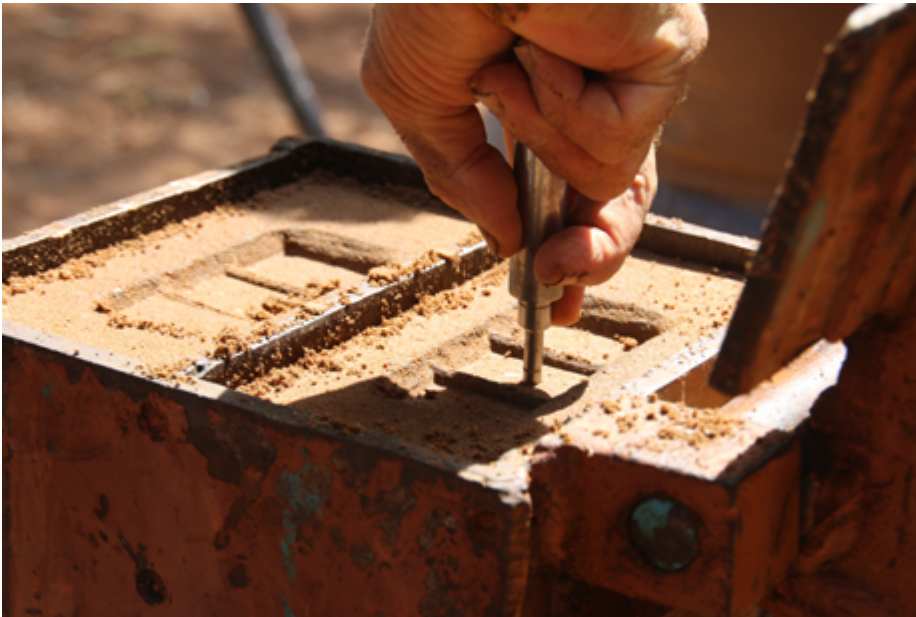
Satprem testing a CSEB in Sri Lanka produced by an old Balram press
