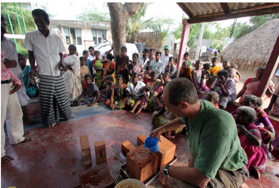
Satprem demonstrating erosion and lack thereof in raw and stabilized earth samples
