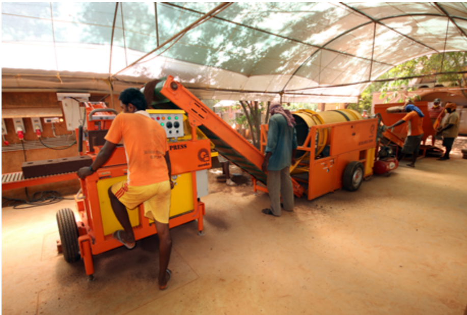
The Auramix 5000 and Auram Press 4000, designed by AVEI and Aureka, producing blocks for the upcoming Sharanam project
