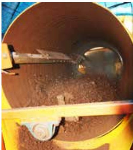
Water being added to the mix in the drum
