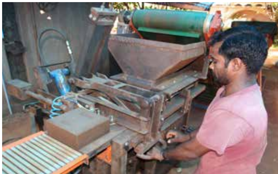
One block being compressed while another waits to be offloaded
