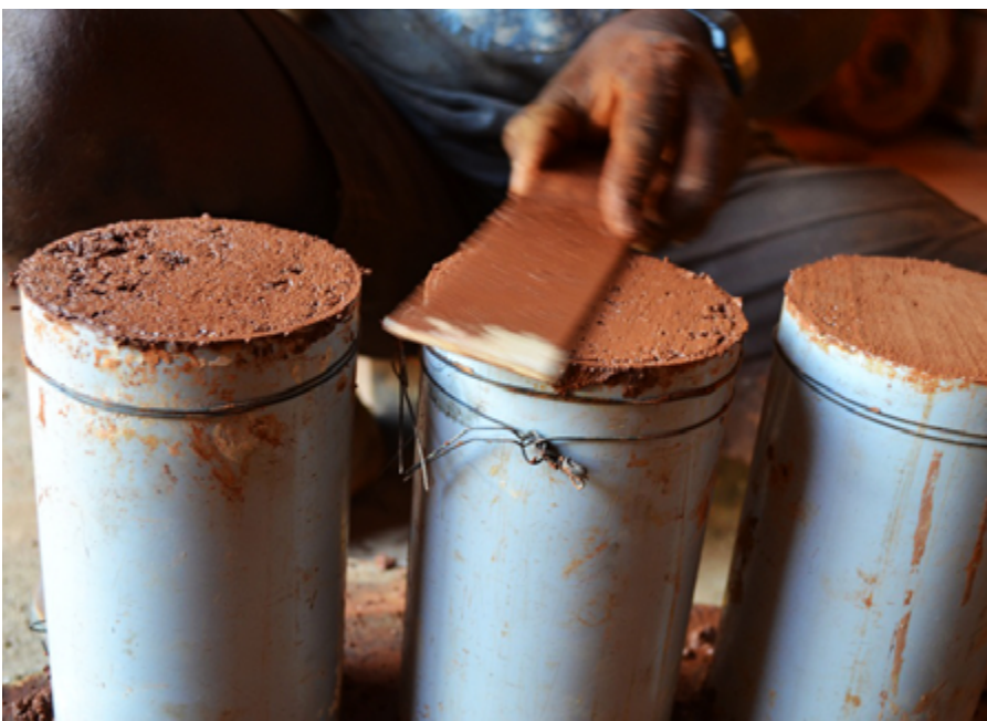
Preparing the cylindrical samples of Poured Earth
