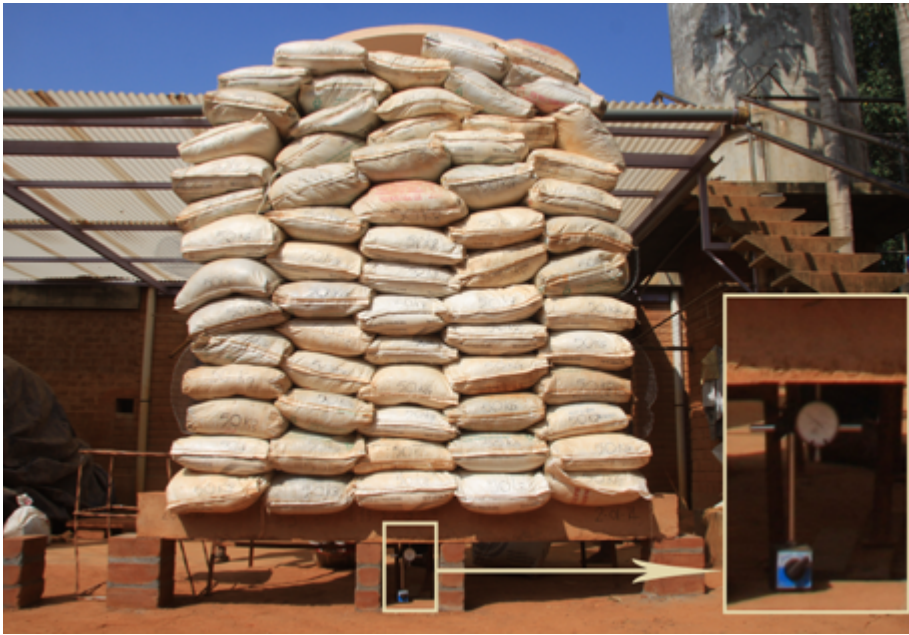
A Poured Earth beam undergoing a flexural strength test
